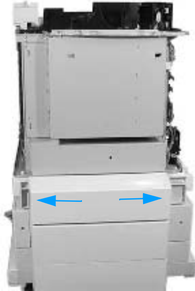
Figure 6-14 Removing and replacing the cassette cover
