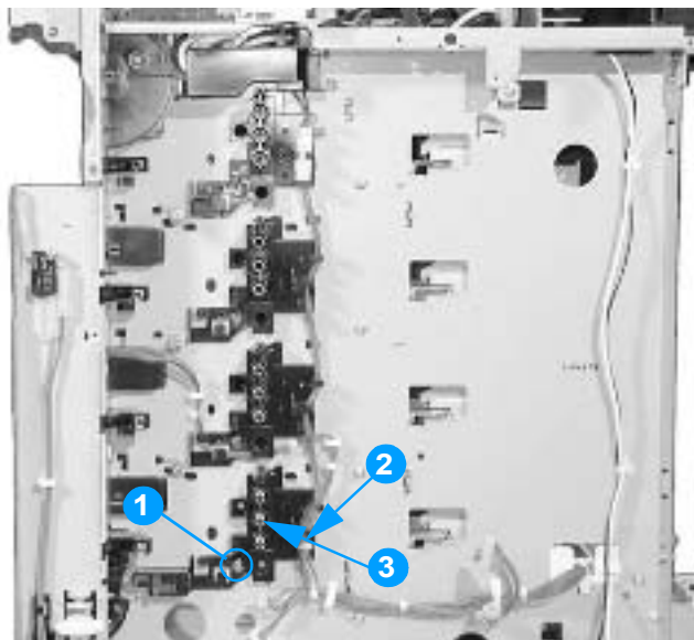
Figure 6-66 Removing and replacing the high-voltage contact blocks (cyan indicated)
