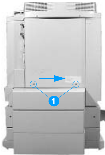
Figure 6-3 Removing and replacing the rear cover
