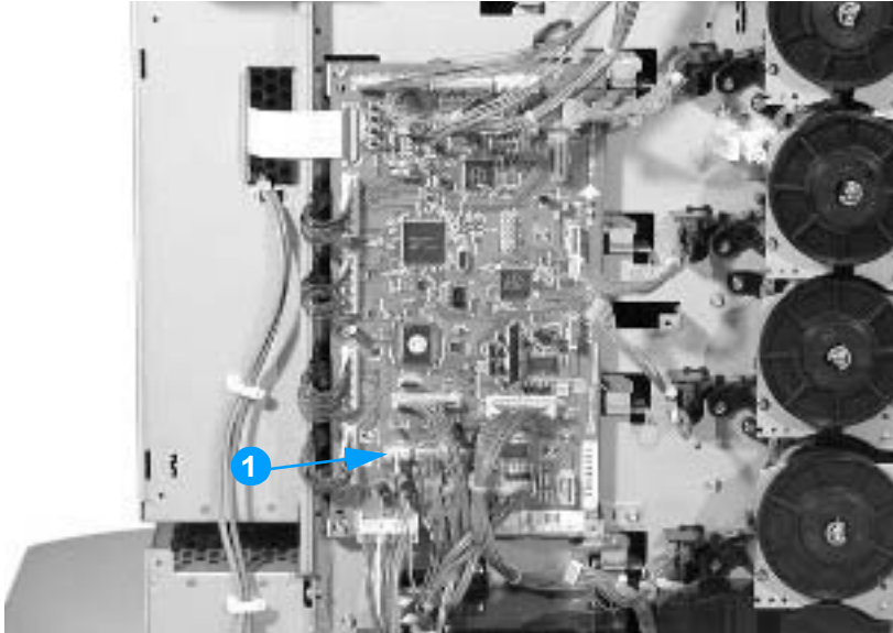
Figure 6-46 Removing and replacing the power supply fan (1 of 2)
